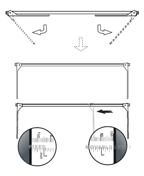
Measurement range is from 65mm to 1000 mm / 2.5 - 39 inches Slide foot-stop to measure the length of baby.
