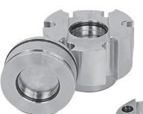
The top and bottom cups are CNC machined and precipitation hardened to a minimum of 40 Rockwell C to allow the integration of DC load cells into a scale that originally used a MTX or PDX load cell. These stainless steel cups maintain the effectiveness of Cardinal Scale's anti-rotation mechanism while working with the MTX or PDX mounting arrangements.
