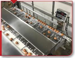
Programmed into the 210 indicator are six preset egg weights determined by the operator.
