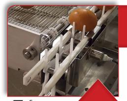
Eggs are optically scanned for placement and weighed, which is read and stored in the 210 indicator.
