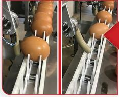
The eggs are then moved along the chain conveyor to "kickers". an implement that pushes the egg off of the chain conveyor—into the grading station determined by their weight.
