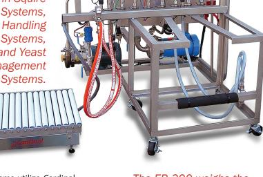
The Grain Handling Systems and Yeast Management Systems utilize Cardinal Scale's 825 or 225 weight indicator and the company's TBCSS1KM-4 load cell kits. The TBCSS1KM-4 load cell kits provide the durability and precision needed to take on filling of grain augers, mills, and hoppers or multi-tank yeast propagation systems. The 825 or 225 weight indicator guides the more complex filling functions associated with the aforementioned tanking systems.
