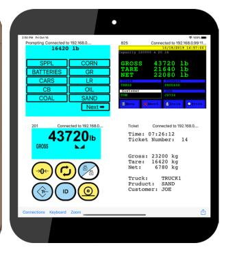
RemoteWeigh makes your iPhone, iPad or iPod touch into a remote control for your Cardinal/ Detecto weight indicators. Up to eight different weight indicators may be connected simultaneously. Real-time updating weight is displayed. Provided functions include zero, tare, gross/net. ID, and change units. RemoteWeigh may be used as an 825 indicator remote control and supports Cardinal prompting protocol.
