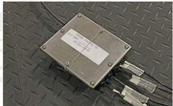
Figure No. 2 Security Seal on Load Cell Junction Box
