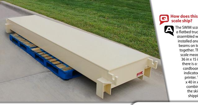
The SWIM scale ships on a flatbed truck. It arrives assembled with load cells installed and the level beams on top all banded together. This skid with the scale measures 165 in x 36 in x 15 in. Additionally, there is a separate cardboard box with the indicator, checkrods, and printer. This box is 48 in x 40 in x 17 in. The total combined weight of both the skid and box is 4,331 lb shipping weight.
