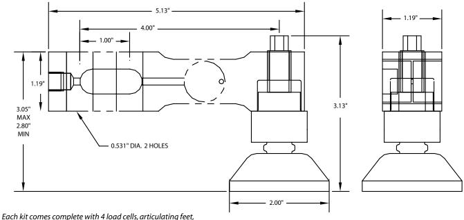
Each kit comes complete with 4 load cells, articulating feet, summation junction box, and 25 feet of load cell cable.
