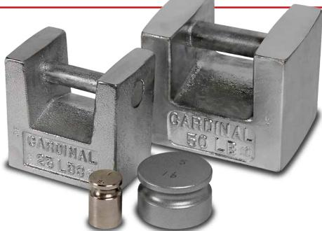
Designed for use in the calibration of scales, Cardinal Scale's test weights have been calibrated using reference standards tested by the State of Missouri Department of Agriculture (**State Test No. 1119 & 1121**) and traceable to the National Institute of Standards & Technology through **NIST Test No. 259883**.
