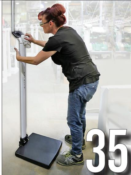
Each of the four load cells in the scale base are calibrated individually. **500-lb test weights** are used to test the icon's accuracy.
