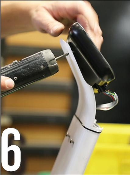
Assembling the indicator to the column and scale base is a streamlined process that minimizes potential production issues. Altogether, an indicator can be **assembled completely in 6 minutes or less** at DETECTO's factory in Webb City, MO.
