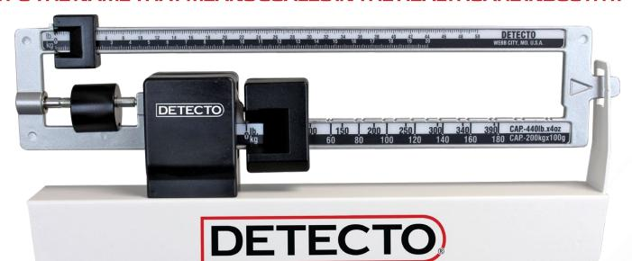
The die-cast weighbeam is easy to read from both sides and makes weighing fast and simple.
