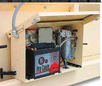
Load cell junction box located inside the battery box for easy access.
