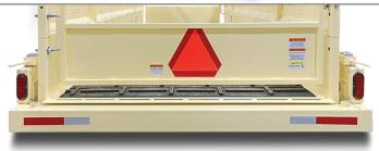
Extra-thick, heavy-duty bumper plates (½" thick).
