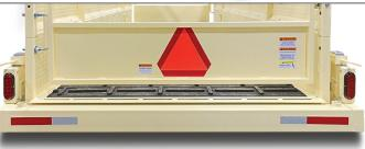
Extra-thick, heavy-duty bumper plates (½" thick).
