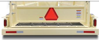
Extra-thick, heavy-duty bumper plates (1/2" thick).
