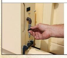
Air purge valve releases air from air bags to easily and quickly lower into weighing mode.
