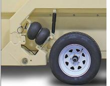
**Industry-leading** standard 15" wheel with 205/75 D rated trailer tire and semigrade airbag suspension.
