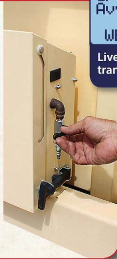
The Weight Wrangler's mobile weighing center includes an inclinometer that eliminates the need to recalibrate the scale after transport. The self-contained scale provides legal-for-trade weights in multiple locations with up to a 5% tilt angle (maximum allowed by NTEP) in any direction.
