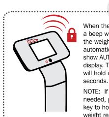
When the weight is stable, a beep will sound and the weight reading will automatically lock and show AUTO LOCK on the display. The weight reading will hold approximately 7
